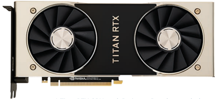
A Titan RTX GPU card; Brains on Board research showed how one of these could equal the performance of 8 custom neuromorphic processor boards from a dedicated brain simulation supercomputer. Image credit: NVIDIA
